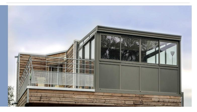
The double-sided technobond panels are part of the CONSERVATORY product range. They are assembled with a self-adhesive hot-melt film based on an extruded polystyrene rubber.
